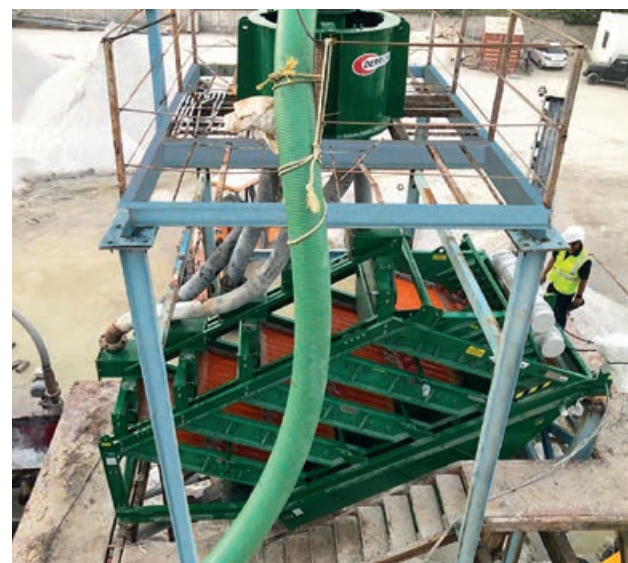
A 5-deck Derrick Stack Sizer fitted with Polyweb panels allows a silica sand plant customer to process 800 metric tons per line each day.
