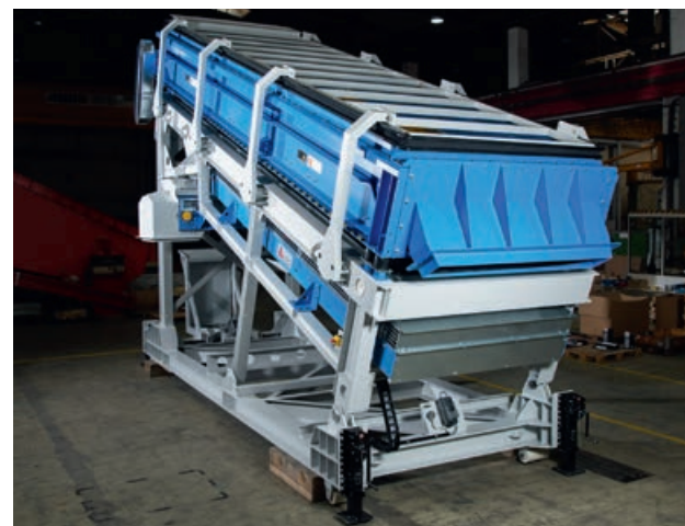
IFE TRISOMAT – the flip-flop screen for difficult-to-handle materials
