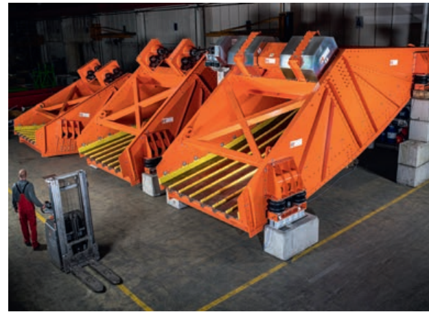
IFE banana screen – ideal for processing material with high contents of fines and high feed rates
