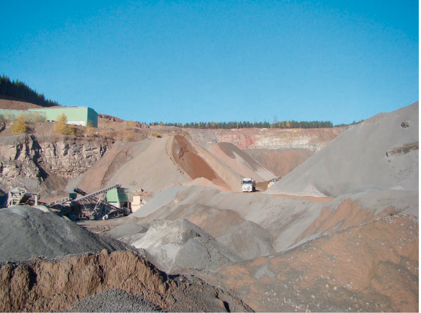
Dumps of crushed sands at a quarry
