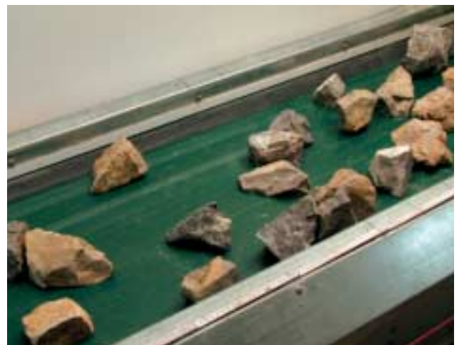
2 Singled limestone particles on a belt conveyor
