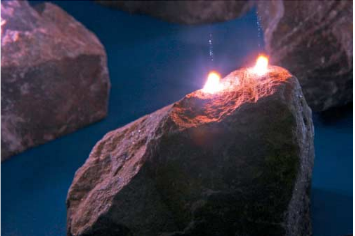
1 Laser-induced plasma on a limestone
