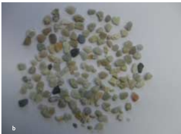
10 Diagram of the cubic (a) and non-cubic fraction (b) of a sorted gravel fraction 4/8 mm
