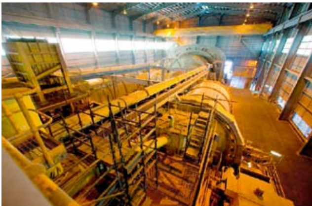
19 Grinding system in a beneficiation plant (Newcrest)
