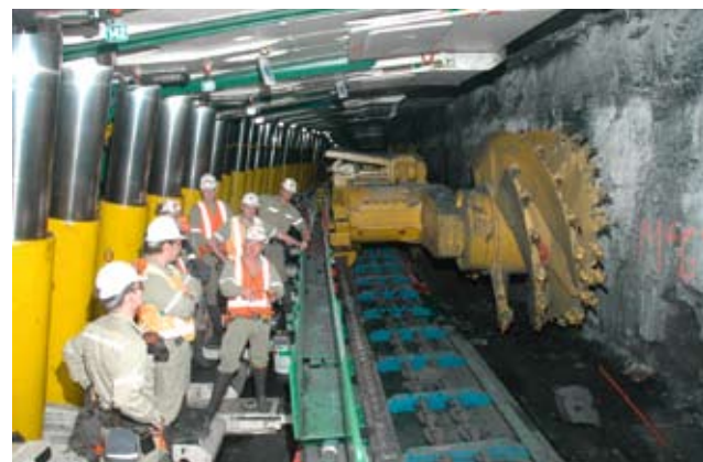
8 Longwall excavation machine at Carborough Downs (Vale)
